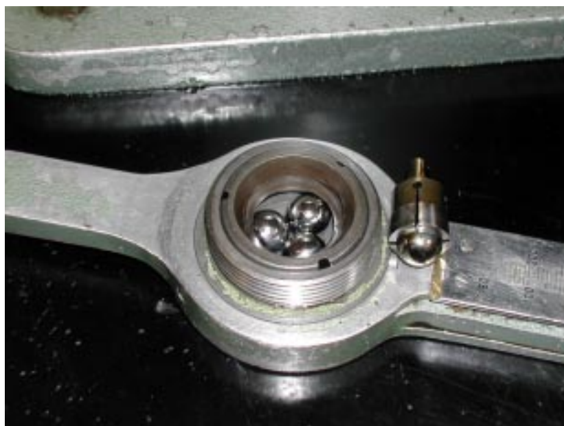
Plate 2: The 4 Balls – Three in the Cup with Clamping Ring and the Third in the Chuck awaiting location within the Spindle.
